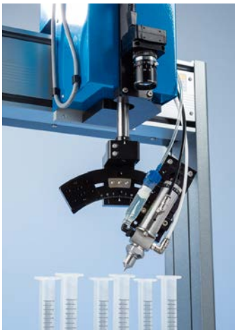
Smart vision CCD camera verifies workpiece presence and orientation.
