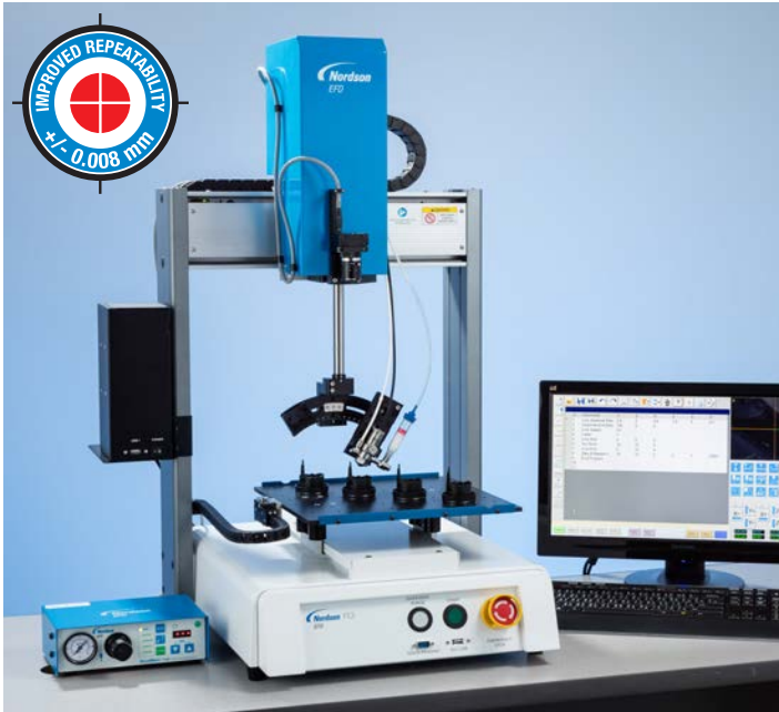
RV Series makes 4-axis dispensing automation more intuitive with proprietary DispenseMotion software.
